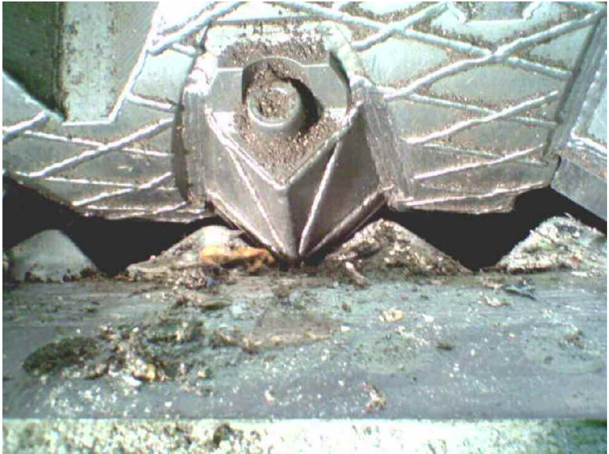
Figure 5 Cutting process rotor knife in stationary knife
