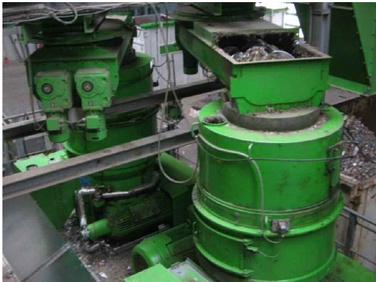
Figure 7 Pelletizing presses with spiral and dosing conveyor
